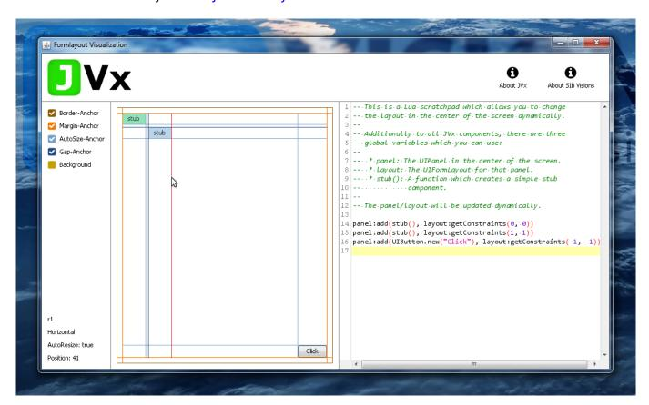
On the left is the possibility to show and hide anchors together with the information about the currently highlighted anchor. On the right is an Lua scripting area, which allows you to quickly and easily rebuild and test layouts. It utilizes the JVx-Lua bridge from a previous blog post and so any changes to the code are directly applied.
