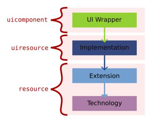
The resource itself, accessed by calling <uiwrapper>.getResource(), is the extension/technology component. The UI resource can be accessed by calling <uiwrapper>.getUIResource(). The UI component can be accessed by calling <uiwrapper>.getUIComponent() and is usually the UI wrapper class itself. If we use our previous Swing example, the resource would be a JVxButton/JButton, the UI resource would be the SwingButton and the UI component would be the UIButton.
