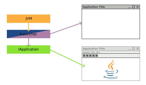
So we need two classes, the ILauncher implementation that knows how to start the technology and the IApplication implementation. That we already knew, so let's try to put this into code. For simplicity reasons (and because I don't want to write a complete factory from scratch for this example), we will reuse the Swing implementation and write a new launcher and application for it.
