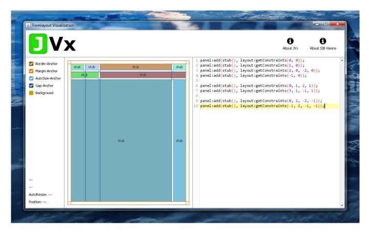
The main difference is that columns and rows are sized according to the components and not given a fixed-width portion of the panel.
