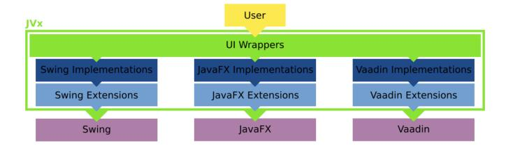
Changing between them can be as easy as setting a different factory. I say "can" because that is only true for Swing, JavaFX, and similar technologies. Vaadin, obviously, requires some more setup work. Theoretically, one could embed a complete application server and launch it when the factory for Vaadin is created, allowing the application to be basically stand alone and started as easily as a Swing application. That is possible.
