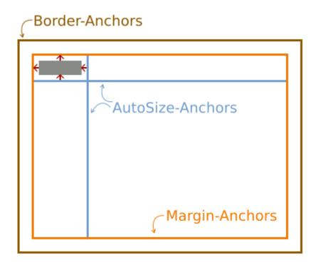
With the coordinates of 0, 0, no new anchors are created. Instead, the component is attached to the top and left margin anchor. Two new autosize anchors (horizontal and vertical) are created and attached to the component.
