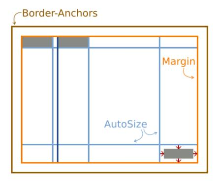
What happens is the same as when adding a component at the coordinates 0,0, except that the reference is the lower right corner. The component is attached to the bottom and right margin anchors with trialing autosize anchors.
