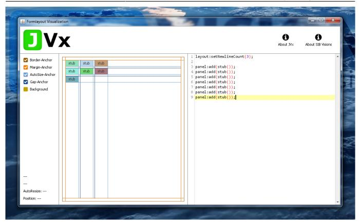
It does not require any interaction from us except adding components. In this case, when three components have been added, the next one will be added to the next line and so on. This is quite useful when all you want to do is display components in a fixed horizontal grid.
